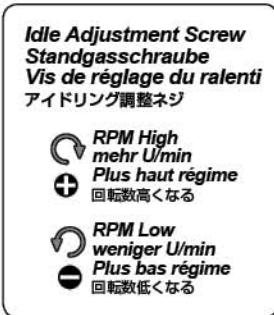
The idle speed is set after the high-speed needle is adjusted and the engine is up to operating temperature. Turn the idle adjustment screw counter clockwise to reduce the idle speed, or clockwise to increase it. The idle speed should be set to not engage the clutch. Set throttle trim to neutral before setting idle.
