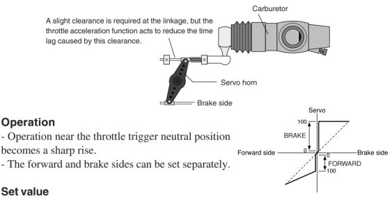
The standard value (100% point) of this setup effects the operation amount set by throttle EPA function.
