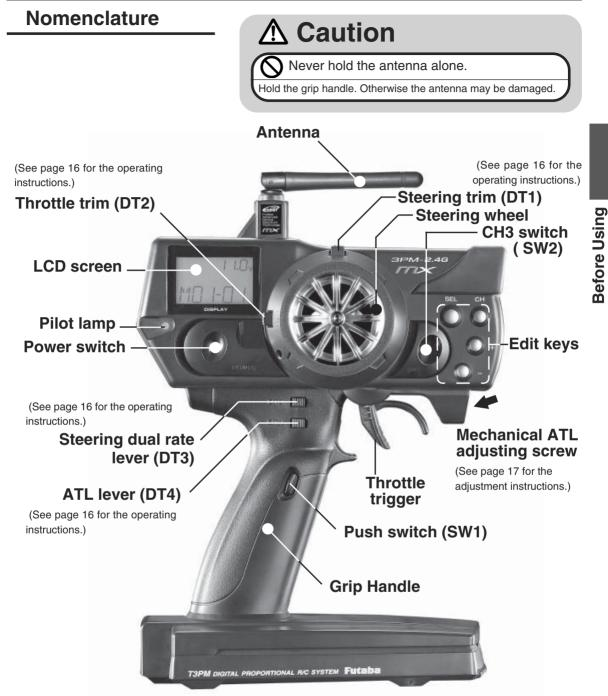
\*The switches and levers in the figure are shown in the initial setting position.
