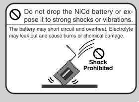
The electrolyte in NiCd batteries is a strong alkali. Should you get even the smallest amount of the electrolyte in your eyes, DO NOT RUB. Wash immediately with water and seek medical attention at once. The electrolyte can cause blindness. If electrolyte comes in contact with your skin or clothes, wash with water immediately.
