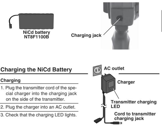
When charging the NT8F1100B NiCd battery with the special charger FBC-19B(4) (for U.S.A.), allow about 24 hours for charging. If the transmitter has not been used for some time, cycle the battery by charging and discharging it two or three times.
