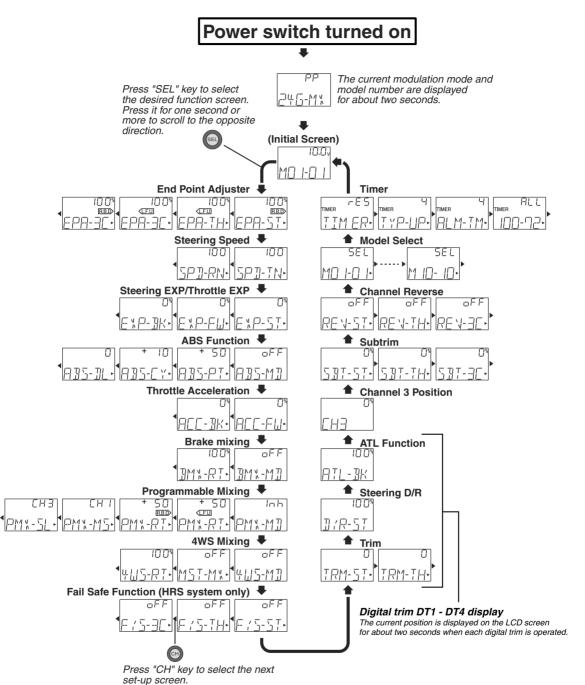
[ABS, BMX, PMX and 4WS] Any set-up screen can not be selected when the function is set to "off" or "inh".
